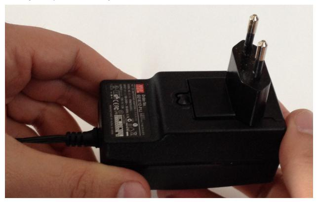
To power-on the board, just connect the external power adapter to Tibidabo connector CN19.
