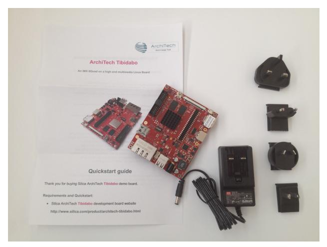
The SPI NOR on the board has been programmed to let Tibidabo boot a *core-image-minimal* image generated with *Yocto*.
